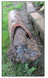
This photo is of a section of a sanitary sewer service line that was removed at a Bremen residence last year because it had become completely blocked with roots and sediment. This exemplifies the type of situation that Columbia Gas encountered at many residences in town.
